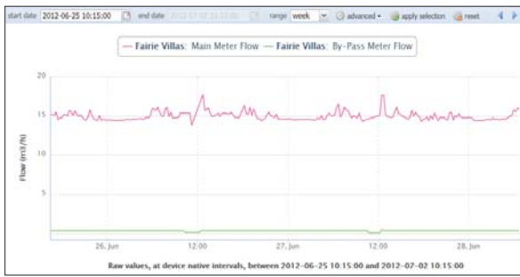
FIGURE 9 Flow logging result into small townhouse complex
